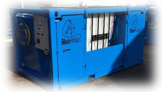
5. Switch on panel. Turn main switch on, Pump 1 On and Pump 2 On. Pump 3 is spare for accessories.
